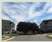
3. This cul-de-sac also has a 50-foot radius but incorporates a vegetated island. This alternative creates about 15% less impervious cover than Option 1.
