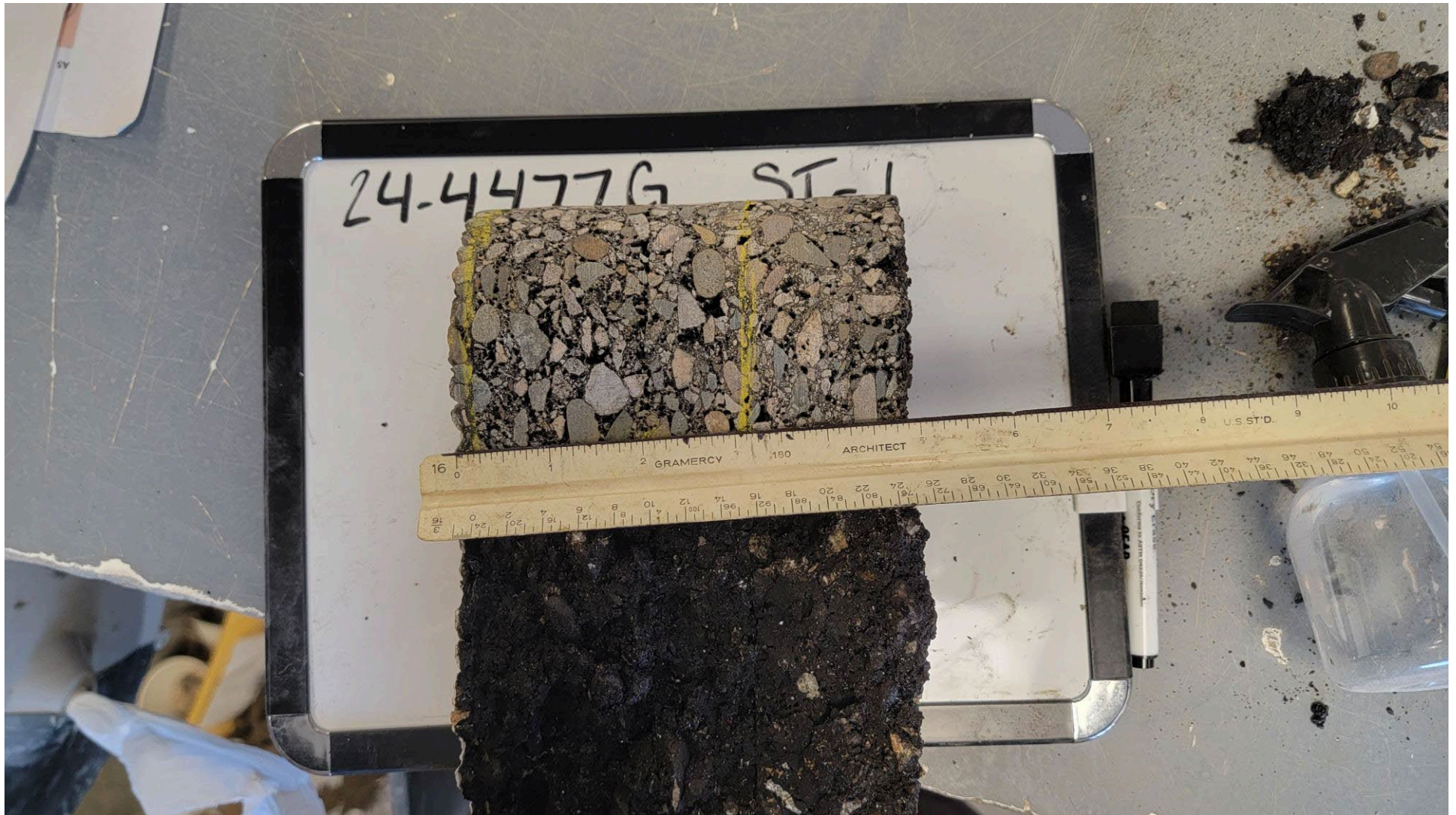
ST-1 Pavement Core, exterior sidewall and interior stripping.
