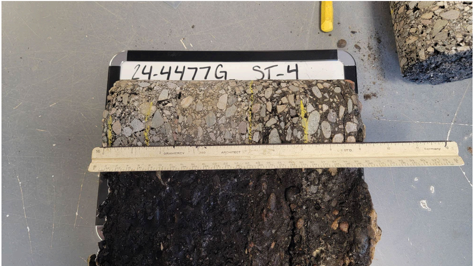
ST-4 Pavement Core, exterior sidewall and interior stripping.
