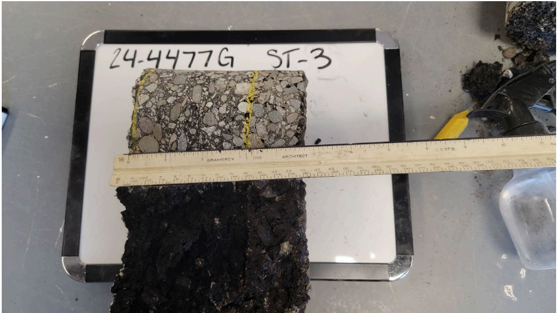
ST-3 Pavement Core, exterior sidewall and interior stripping.
