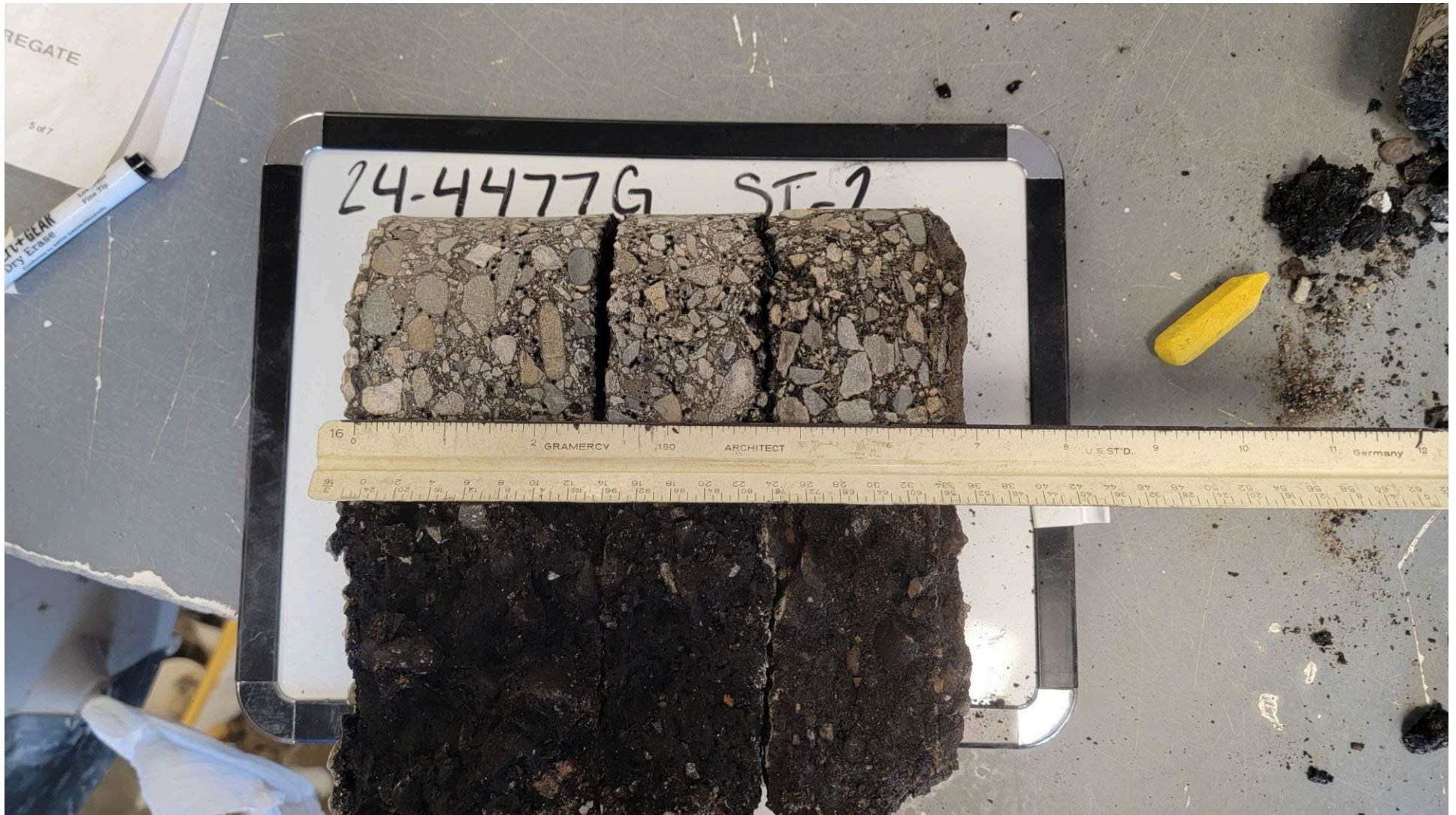
ST-2 Pavement Core, exterior sidewall and interior stripping.
