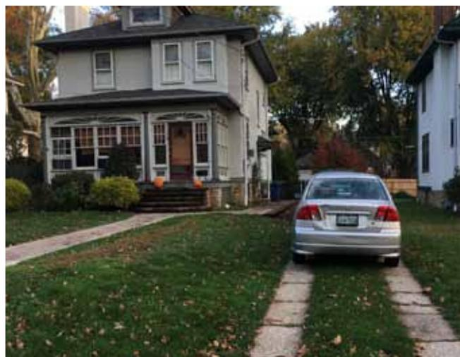
Figure 12. A "two-track" driveway is another way to reduce driveway imperviousness
