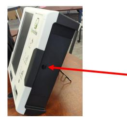
6. When the ExpressVote<sup>®</sup> is configured on a standard table, secure the rear USB port by affixing a tamper-evident label seal as noted below in the photo.
