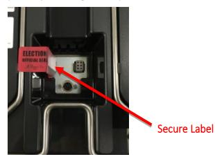
7. Ensure that the access door to the printer transport (on the front of the unit) is closed and locked with the medium barrel key to prevent access to the printing path.
