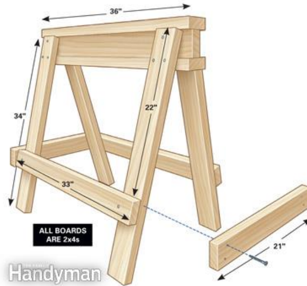
Figure I-3i: Suggested design for sawhorse legs
