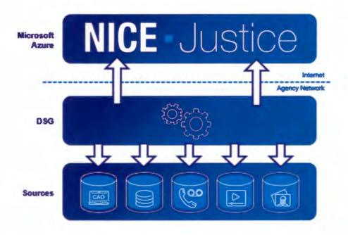
Figure 1 - High Level Architecture Overview
