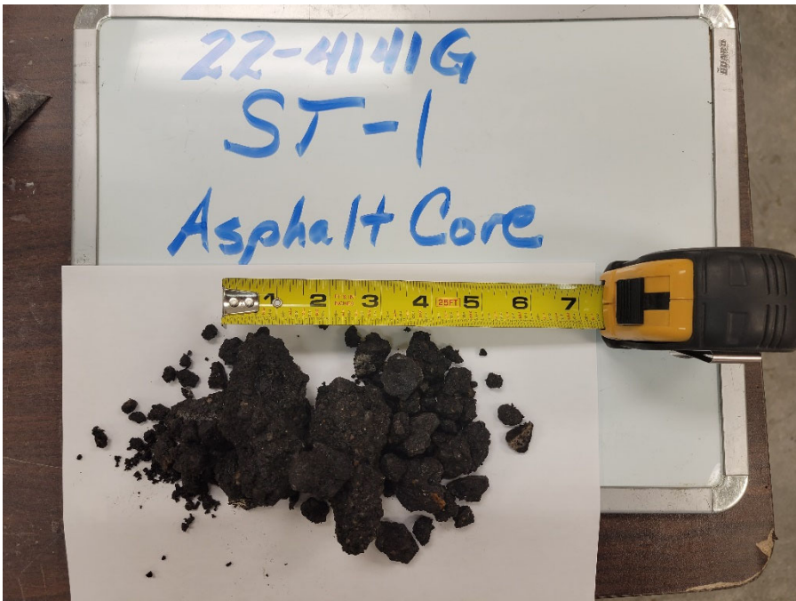
Boring ST-1, Asphalt Core, Cold Mix.
